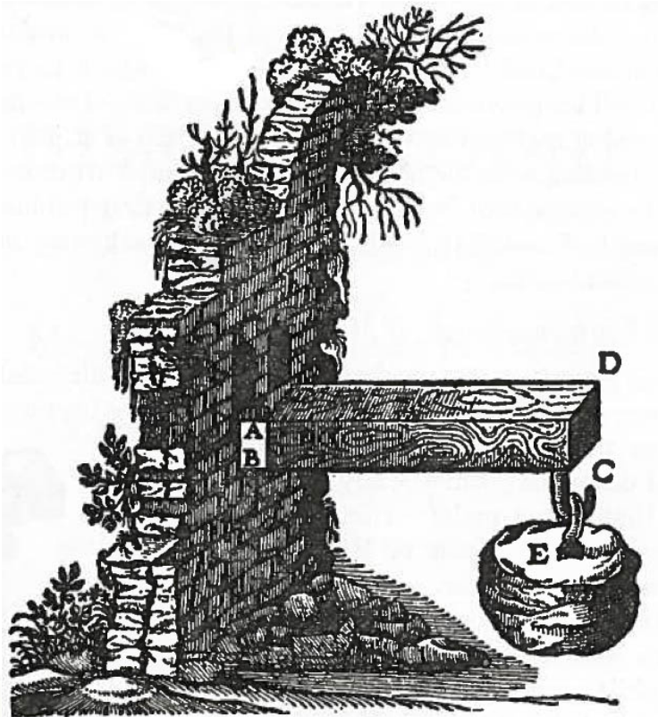
FIG. 15. Galileo's illustration of bending test.
